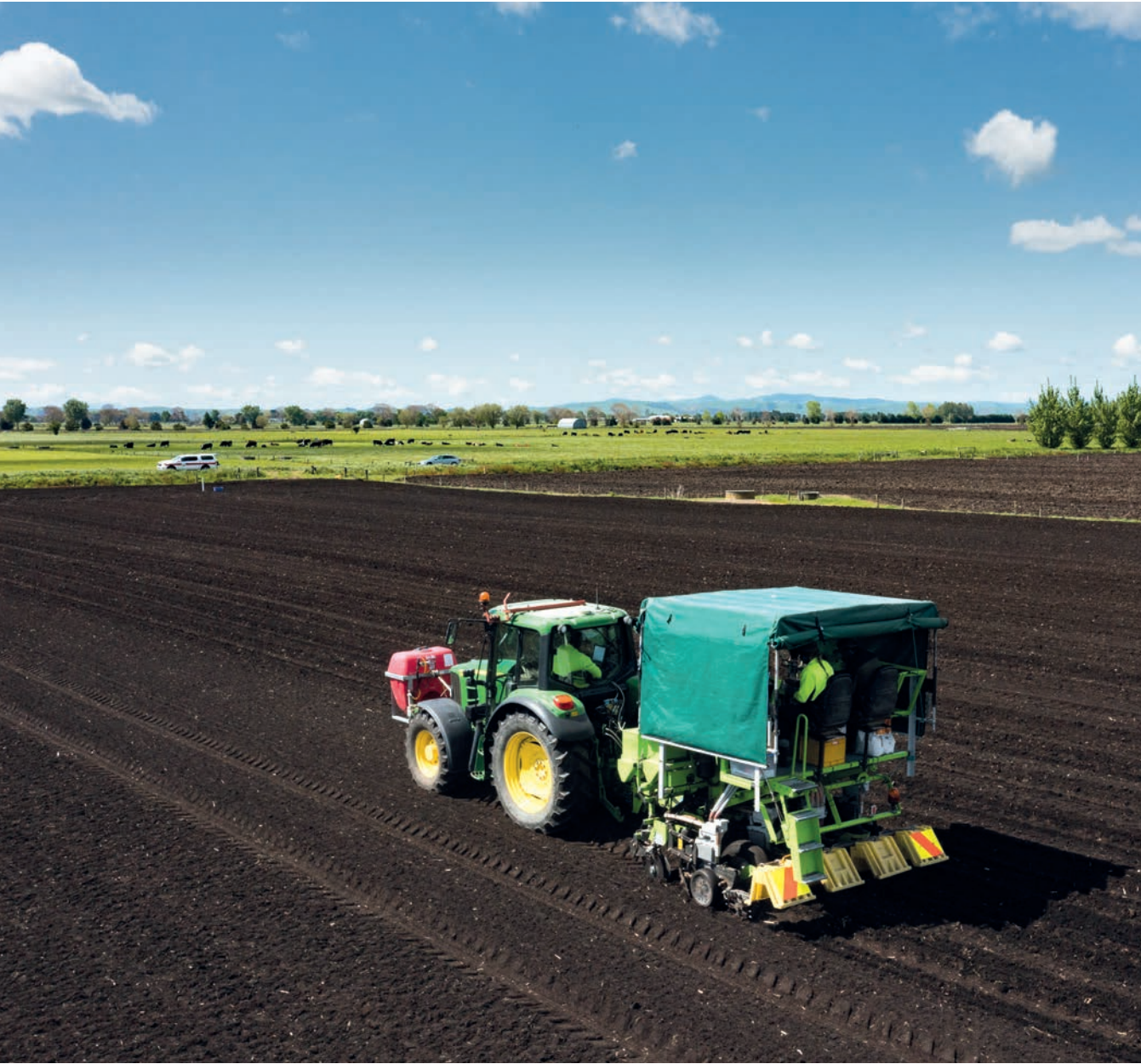
An IMPACT™ small plot planter at Gordonton, Waikato. IMPACT is the acronym for “intensively managed product advancement and characterisation trials”.
